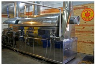
To cook all the sap they collect, the Hering's have a 4 x 14 foot evaporator (*image above*). It uses diesel fuel. To increase efficiency they use a reverse osmosis machine (*image below*). In addition, their evaporator also has a pre-heater unit.
